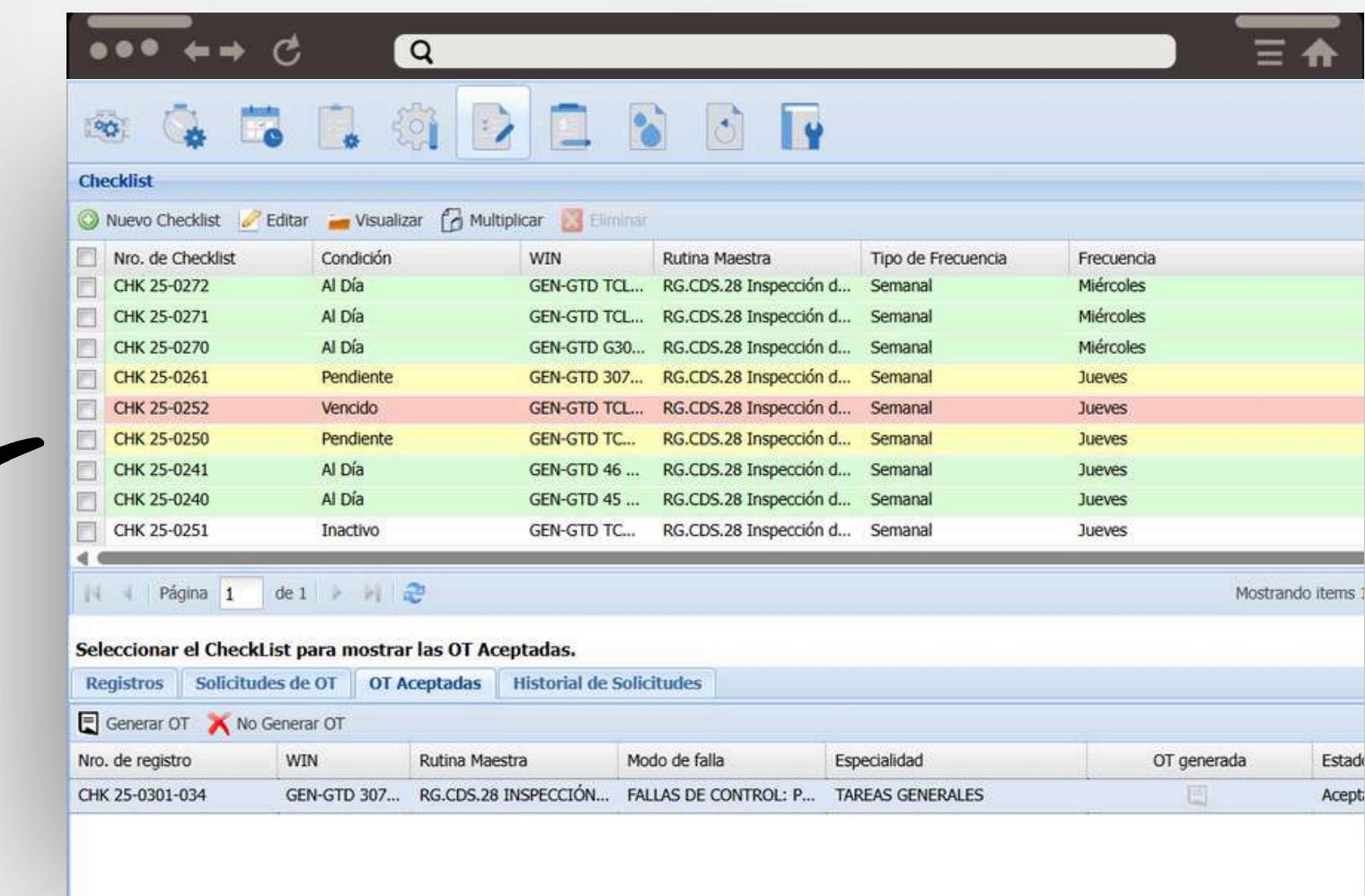
The screenshot shows the 'Checklist' module. It features a table with columns: Nro. de Checklist, Condición, WIN, Rutina Maestra, Tipo de Frecuencia, and Frecuencia. The table lists multiple checklists, each associated with a specific location (WIN), a master routine (Rutina Maestra), and a frequency (Frecuencia). A message at the bottom says 'Seleccionar el Checklist para mostrar las OT Aceptadas.'
